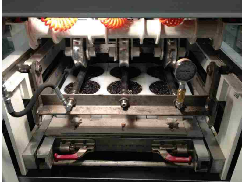
Figure 3.20 - APA Rut Test Setup
