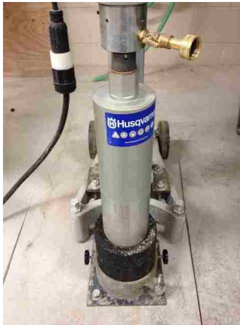
Figure 2 - Specimen Secured in Bottom Jig
