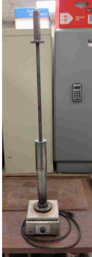
Figure 2 – Compaction Hammer on Hot Plate
