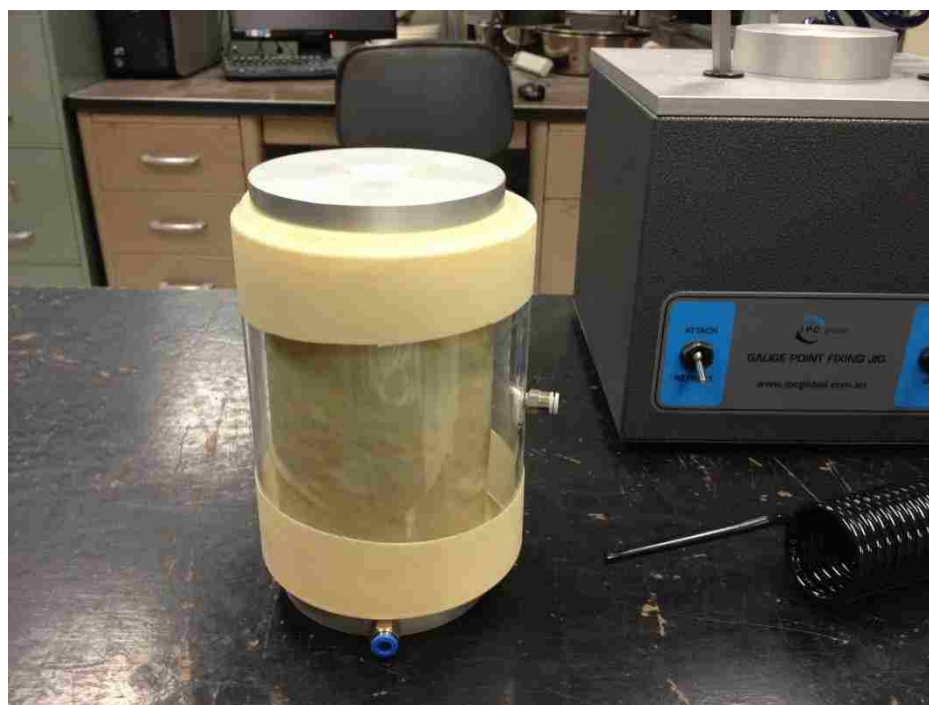
Figure 2 – Collar/Membrane Over Specimen with Vacuum Released
