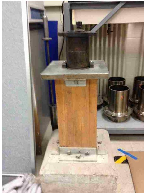
Figure 3.38 - Marshall Compaction Pedestal with Mold Secured in Place
