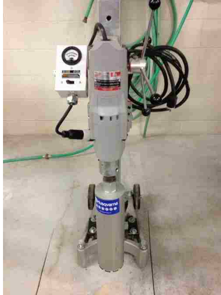
Figure 3.16 - Milwaukee Dymodrill Coring Drill
