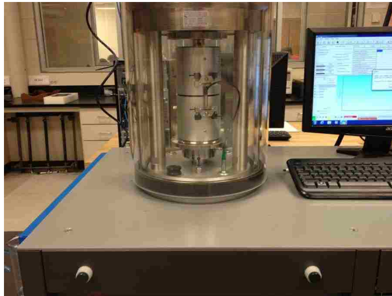
Figure 3.22 - AMPT Test Chamber with Verification Apparatus
