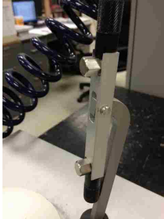
Figure 1 - Fixing Jig Arm with Gauge Points Secured
