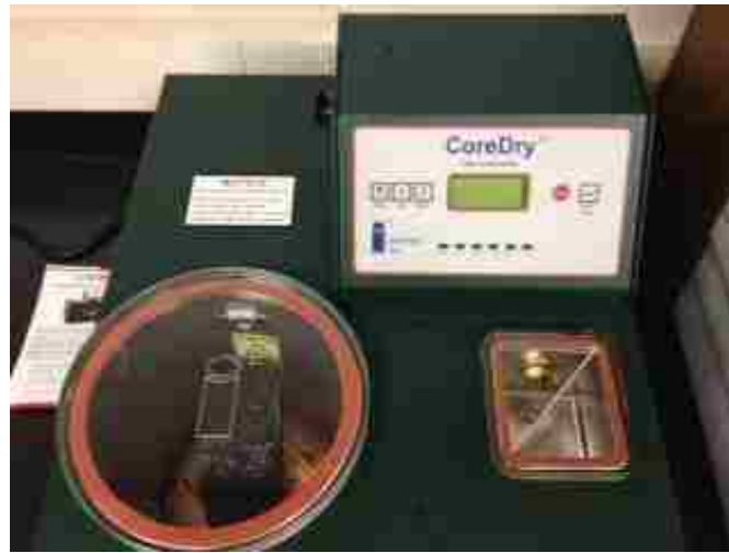
Figure 3.34 - CoreDry Vacuum Chamber
