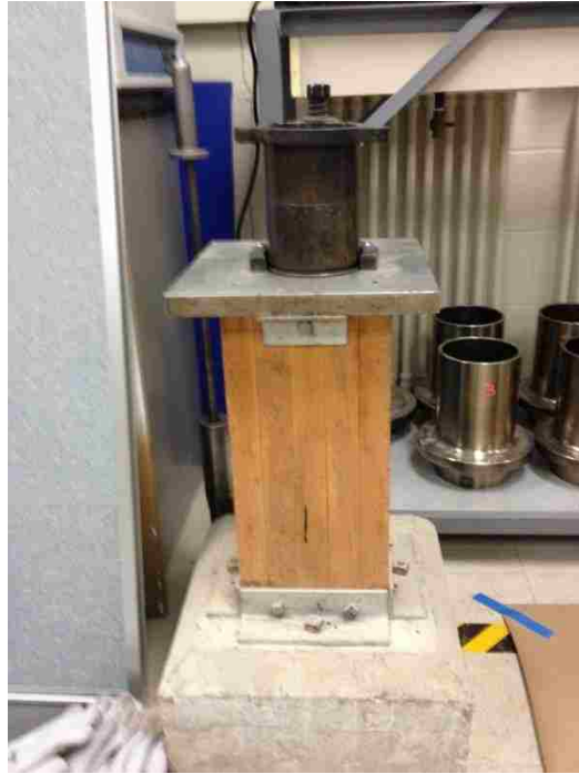
Figure 3 – Mold Secured in Compaction Pedestal
