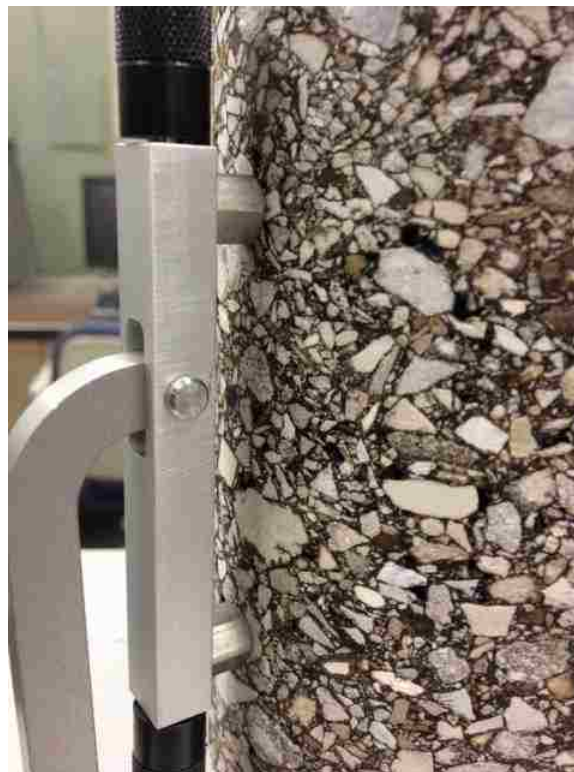
Figure 2 - Fixing Jig Arm Secured Against Specimen Side
